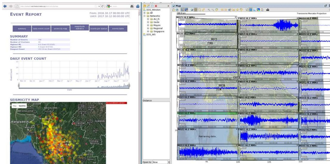
The seismic data is transferred real time by 3G telemetry to servers in Singapore and Nay Pyi Taw, Myanmar (Source: EOS)
