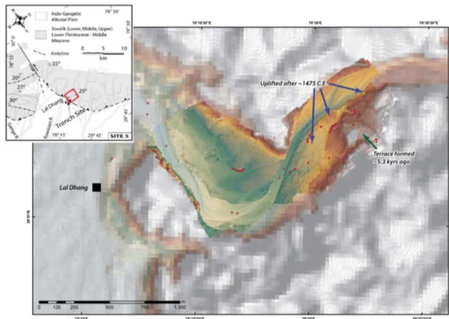
**Figure 6** 0.1 m-resolution Digital Terrain Model generated from drone photographs at Lal Dhang, showing uplifted fluvial terraces along either side of river. Colour code from light-green to white shows increasing elevation. Location map (top left) is from Kumar et al. (2006).
